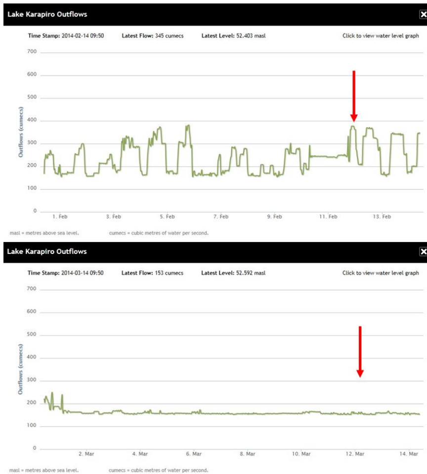
Figure 8: Time series discharge data from Lake Karapiro preceding the February (upper) and March (lower) sampling days (red arrows). The discharge hydrographs show rapid changes in flow under 'normal' operating conditions in February, but very steady flows under the low flow conditions in March. Images are screen grabs of the 7-day discharge charts on the Mighty River web page.
