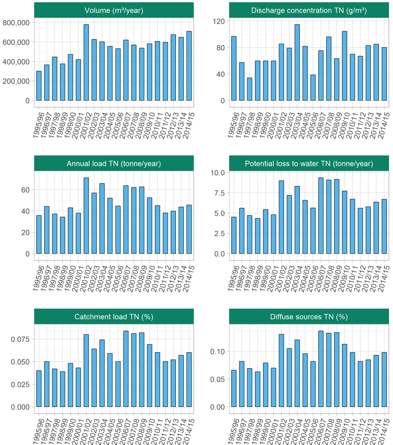
Figure 16: Lichfield wastewater discharge annual volume and TN characteristics (discharge concentration, total annual load applied to land, estimated potential loss to water, % of total Waikato River catchment TN load and % of the Waikato River catchment TN load attributed to diffuse sources.
