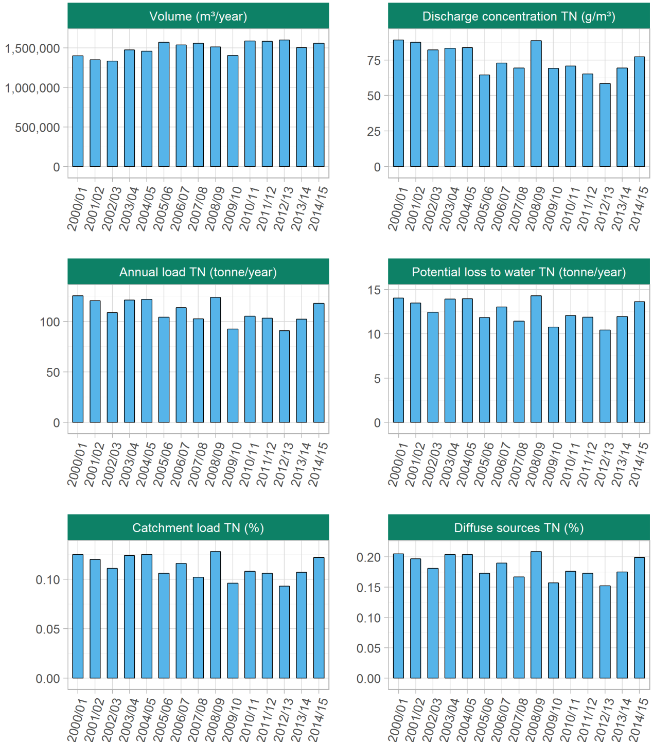
Figure 18: Hautapu wastewater land irrigation annual volume and TN characteristics (discharge concentration, total annual load applied to land, estimated potential loss to water, % of total Waikato River catchment TN load and % of the Waikato River catchment TN load attributed to diffuse sources).
