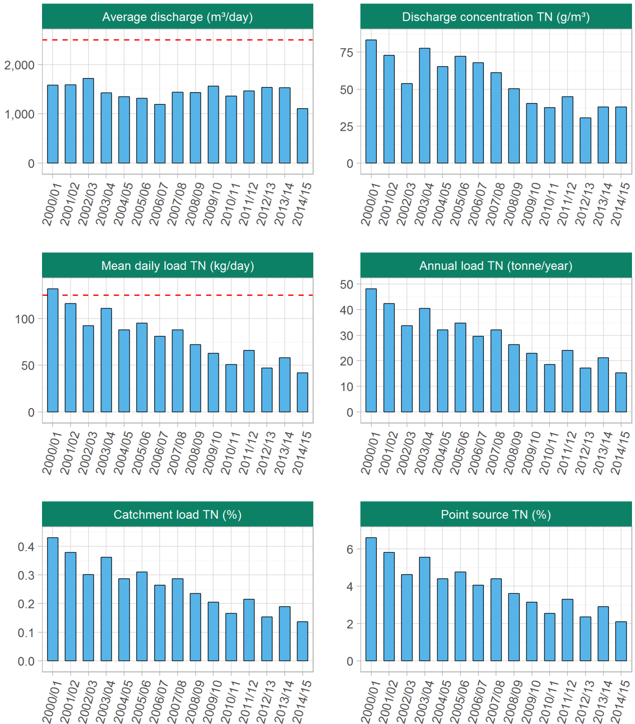
Figure 20: Hautapu wastewater discharge to water average daily discharge and TN characteristics (discharge concentration, mean daily load, total annual load, % of total Waikato River catchment TN load and % of the Waikato River catchment TN load attributed to point sources. Red dashed lines are consent limits.
