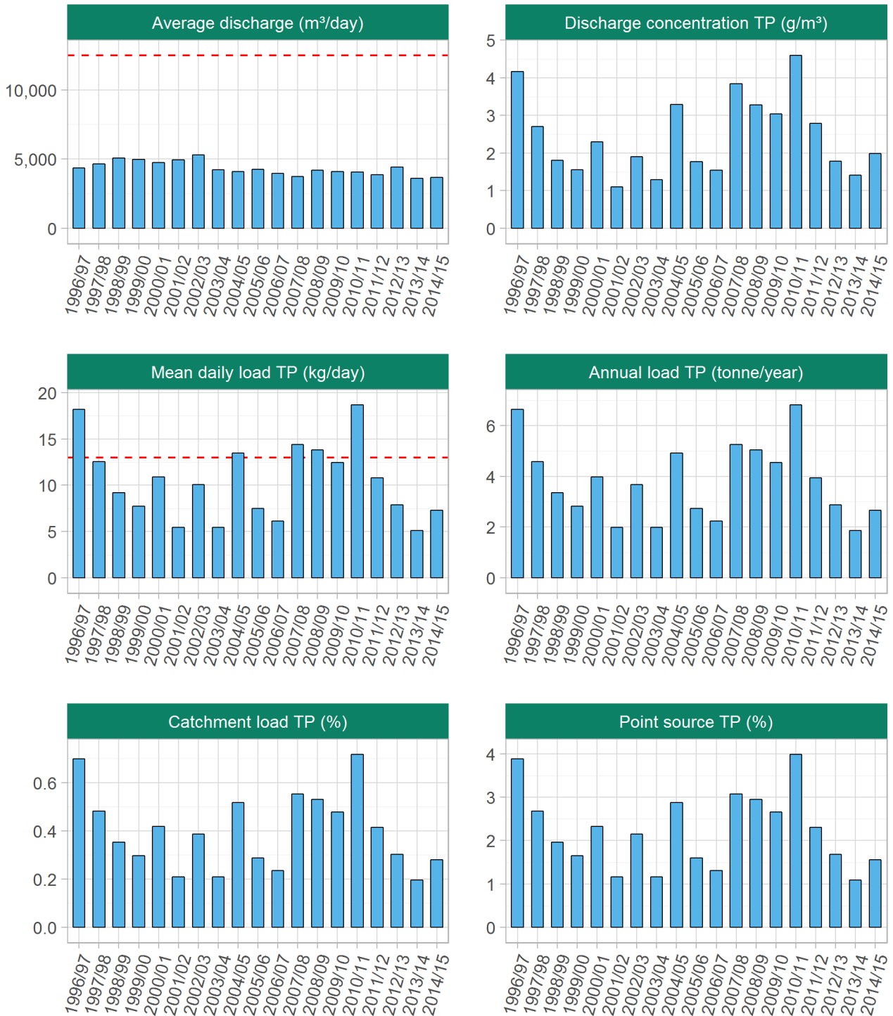
Figure 23: Te Awamutu wastewater discharge to water average daily discharge and TP characteristics (discharge concentration, mean daily load, total annual load, % of total Waikato River catchment TP load and % of the Waikato River catchment TP load attributed to point sources. Red dashed lines are consent limits
