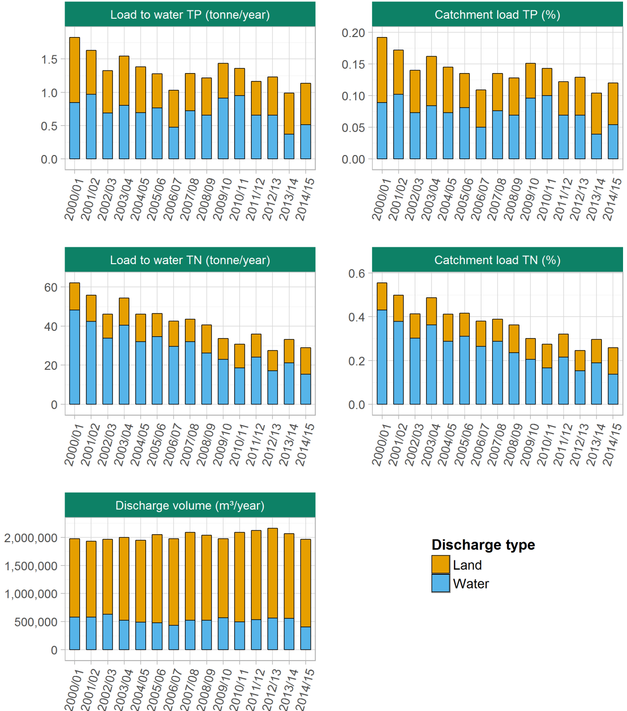
Figure 6: Estimated nutrient loads to the Waikato River, % of catchment load and discharge volume for the water and land discharges from the Hautapu manufacturing site for the period 2001 to 2015.
