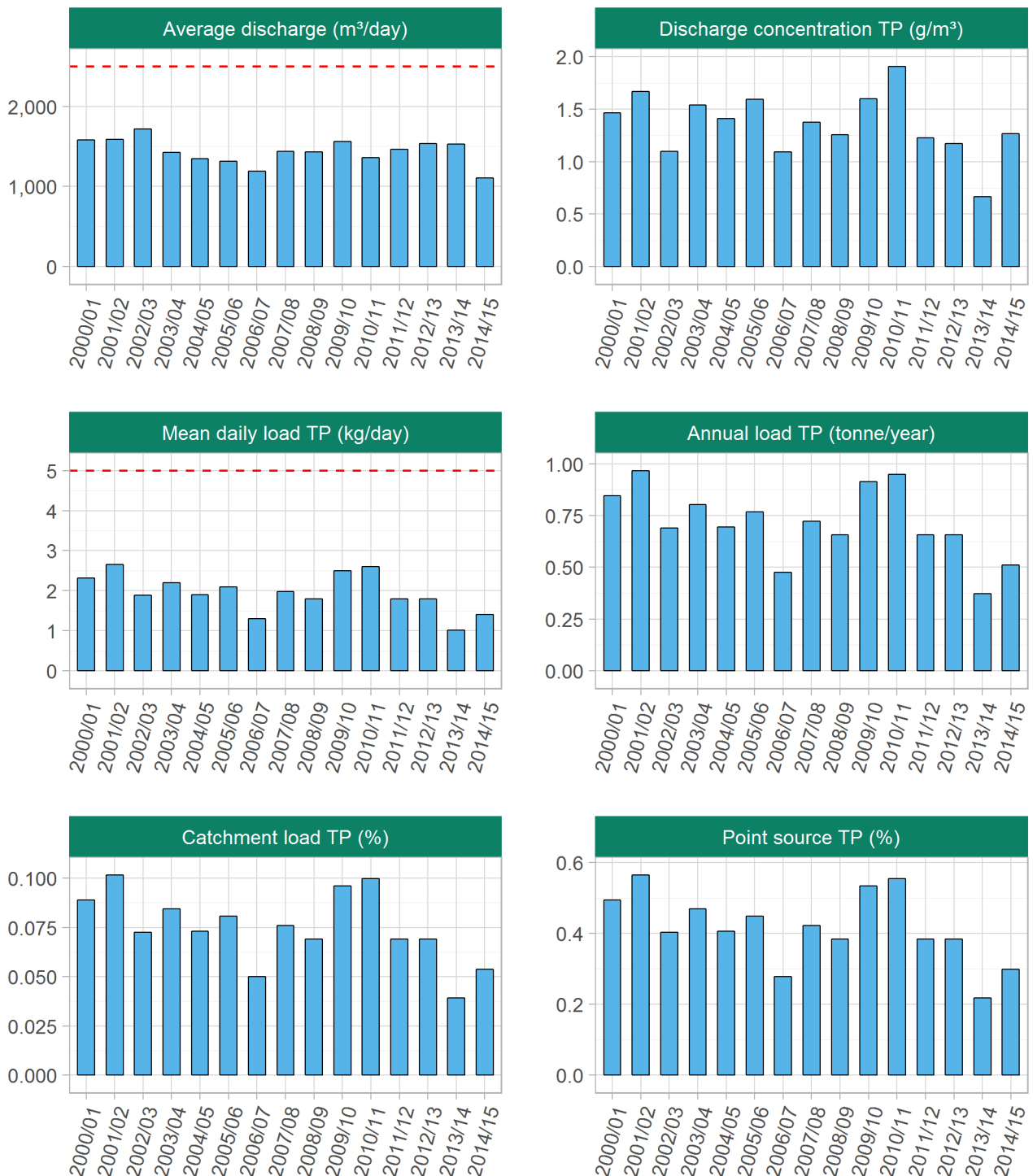
Figure 19: Hautapu wastewater discharge to water average daily discharge and TP characteristics (discharge concentration, mean daily load, total annual load, % of total Waikato River catchment TP load and % of the Waikato River catchment TP load attributed to point sources. Red dashed lines are consent limits.
