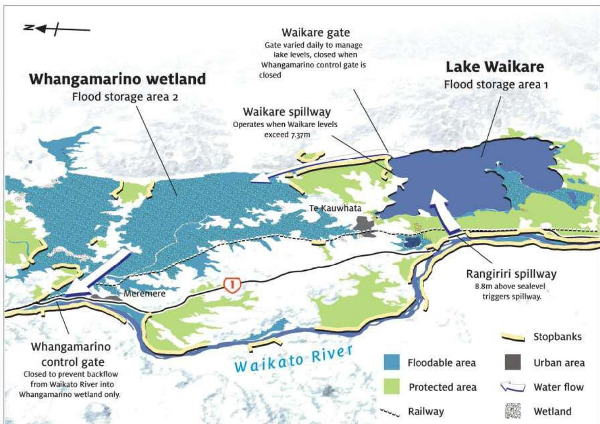
**Figure 1:** Lower Waikato flood protection scheme
