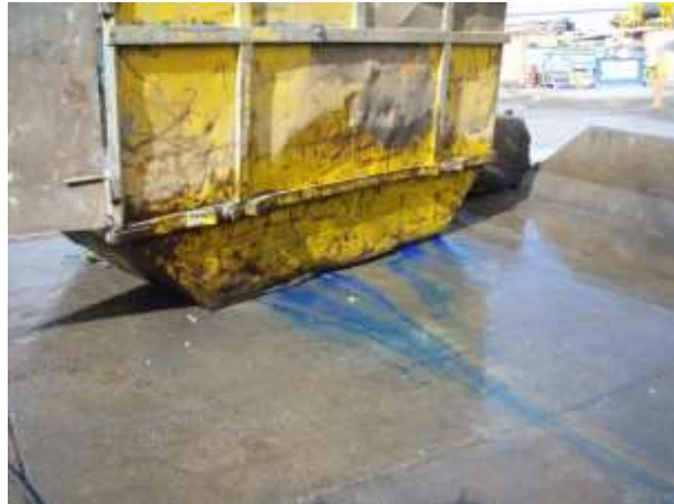
Bin leaking paint into the stormwater system
