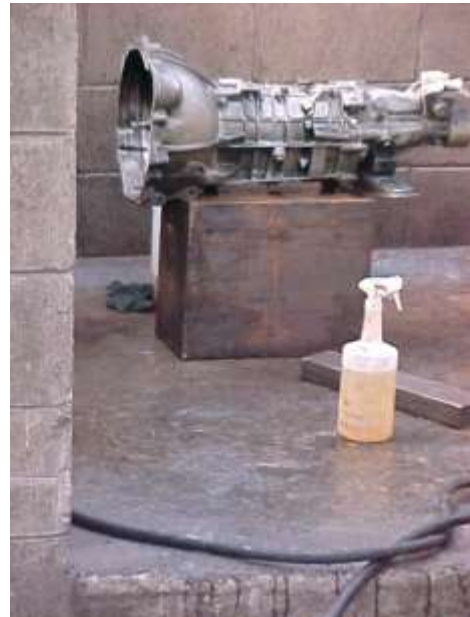
Degreasing where runoff can enter the stormwater system
