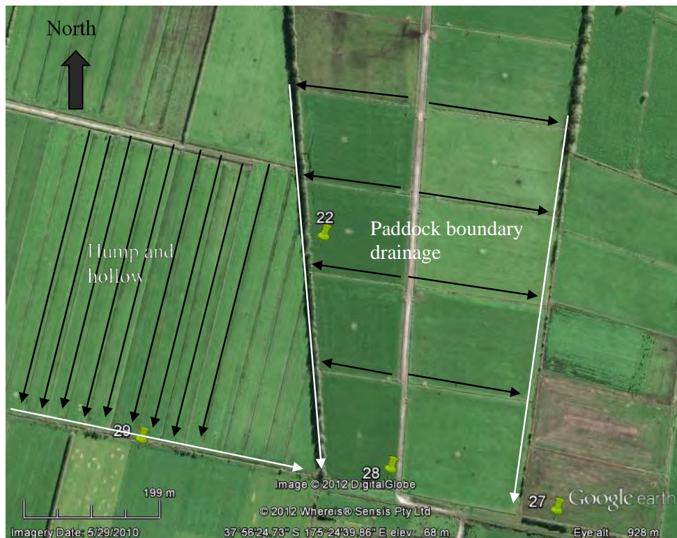
Figure 4. Typical peatland drainage layout showing the contrast between hump and hollow (left side of image) and paddock boundary drainage (right side of image) (image from Google Earth of Moanatuatua peatland). Arrows show drain location and flow direction.
