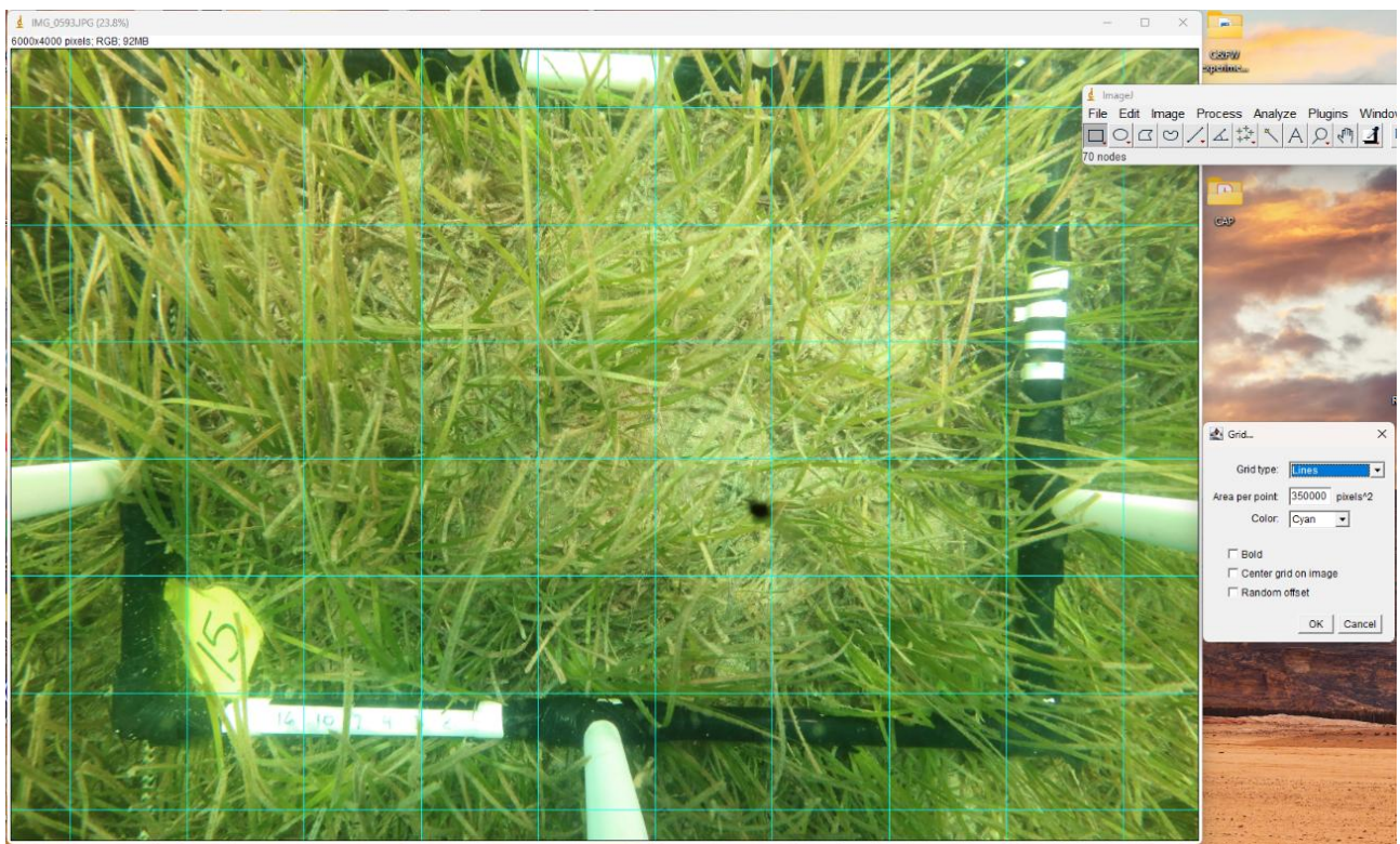
Figure 3. Image showing how seagrass percent cover was calculated using the Grid tool in the ImageJ application. A 6 \times 8 grid was overlaid on a photo-quadrat ( 0.25 \text{ m}^2 ) image and the number of intersections with seagrass was divided by 48 (total intersection points) and multiplied by 100.
