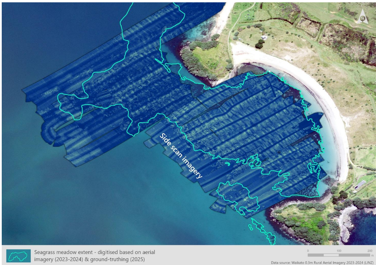
Figure 5. Imagery of side-scan sonar of South Bay (south), and southern section of Stingray Bay (north), Slipper Island / Whakahau, provided by BlueBoat, with estimates of seagrass meadow extent from the 2025 survey (solid green polygons). Note that the texture change of side-scan imagery matches the boundary estimated by ground-truthing extent of seagrass from aerial imagery.
