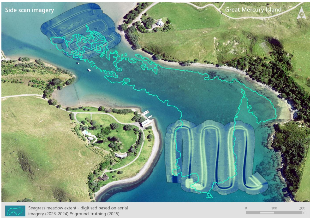
Figure 7. Imagery from side-scan sonar of northern and southern extent of seagrass meadow in Huruhi Harbour, Great Mercury Island/ Ahuahū, provided by BlueBoat. Estimates of seagrass meadow extent from the 2025 survey are displayed with solid green polygons.
