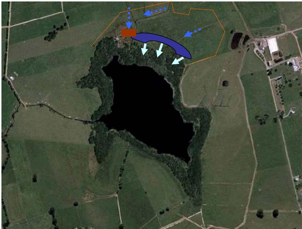
**Figure 28:** Aerial photograph (Environment Waikato) showing the location of the potential fence line (orange dotted line), inflow of drain water (blue dotted arrow), woodchip area (brown square), infiltration filter system (solid blue arch, not to scale) and dispersion of filtered water (blue solid arrow) into Lake Mangahia.
