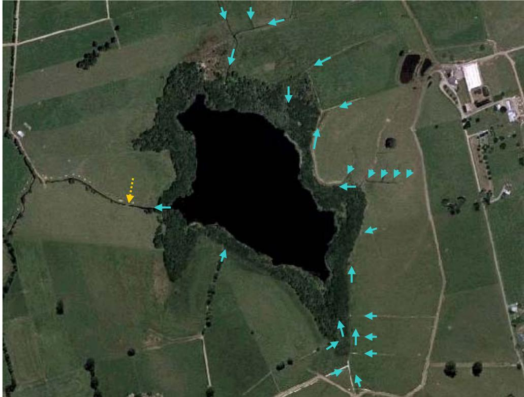
**Figure 26:** Aerial photograph (Environment Waikato) of Lake Mangahia. Aqua arrows indicate the water flow directions of drains, inflows and one outflow. The weir location is shown by the yellow dashed arrow.
