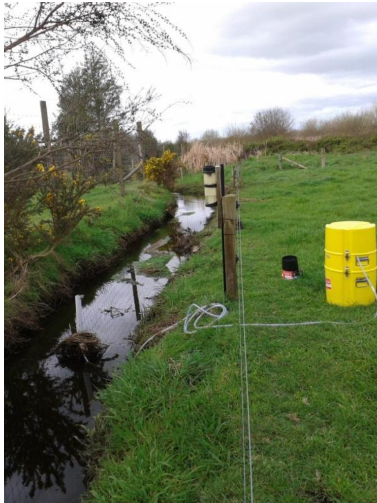
Figure 5. Manning automatic sampling equipment deployed at Rotopiko South 02.
