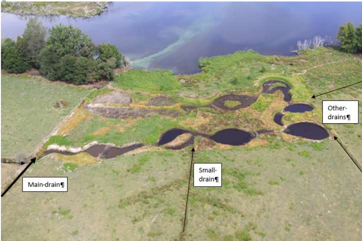
A constructed treatment system at Lake Mangakaware that consists of a series of silt traps and infiltration wetlands. This CTS treats the main inflow and several smaller drains. A green algal bloom can be seen in the lake. (Photo: copyright Waipā District Council)
