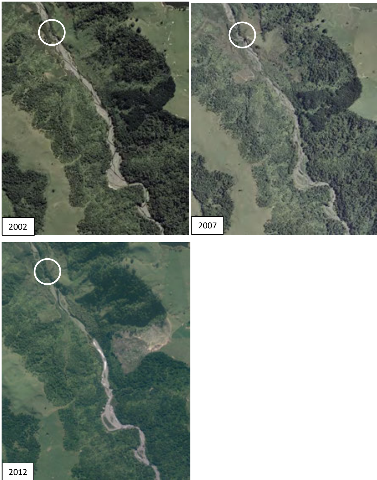
Figure 4-5: Aerial photographs showing changes in the reach downstream of the ignimbrite gorge. Note flow is from bottom to top. The circled area indicates the location of the bedrock pinch.
