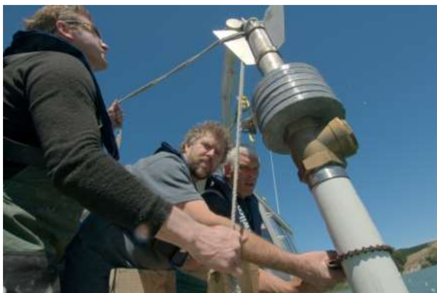
Figure 2-5: Sediment coring from R.V. Rangitahi III. Retrieving a Gravity Corer used to collect sediment cores in the Firth of Thames (photo: Rod Budd, NIWA, Hamilton).
