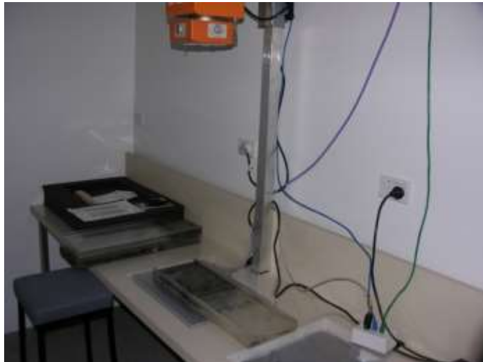
Figure 2-6: NIWA digital x-ray system, with a sediment slab mounted on the detector plate ready for imaging. (Photo: Ron Ovenden, NIWA Hamilton).
