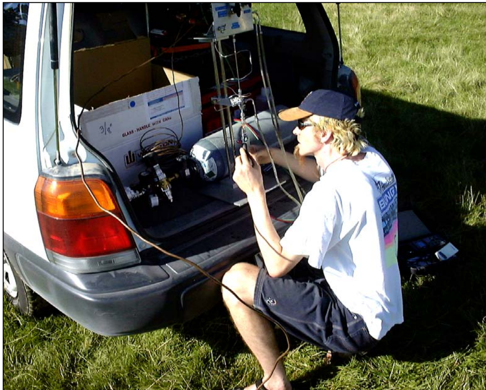
Plate 4: Water sampling for CFC dating
