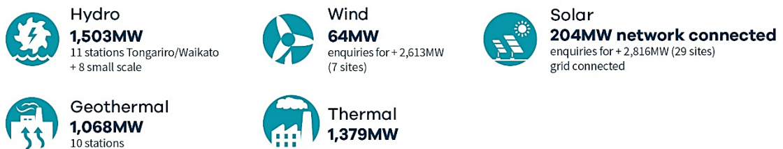
Figure 4: Waikato’s electricity supply (2024)
